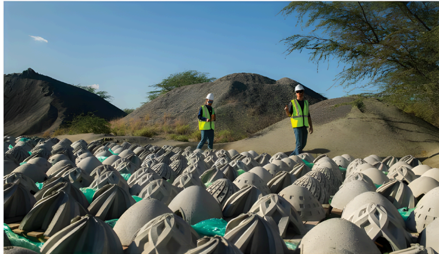
Fake it 'til they make it: The R3D team tested more than a dozen substrates for the hybrid reef before landing on concrete. "Everything from Quikrete from Home Depot, to Hardie Board, limestone and basalt," says project manager Ben Jones. Above, Josh Levy (right) and Ayrton Medina count the R3D project's coral growth modules at the precast yard in Kapolei.
